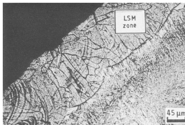
Figure 1 Cross-section of LSM zone for specimen CO1. Electrochemically etched in 10% chromic acid.
