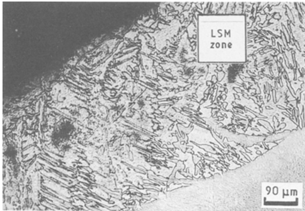
Figure 5 Cross-section of LSM zone for specimen ND2. Electrochemically etched in 10% chromic acid.
